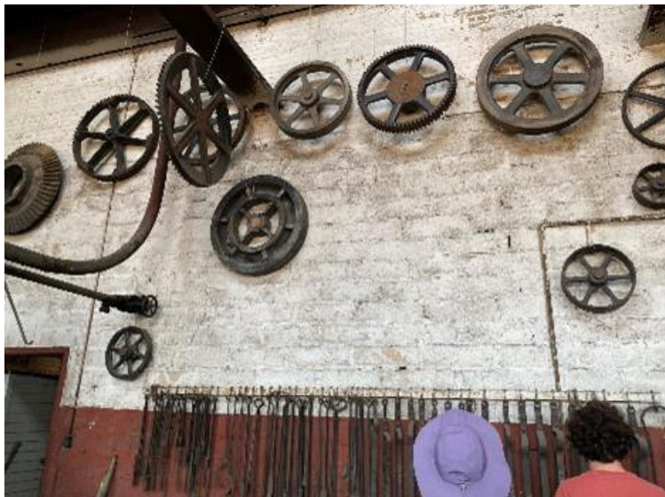
Old wooden patterns were used to make gears.
